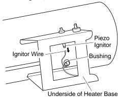
Figure 17 - Removing Ignitor Wire from Piezo Ignitor
